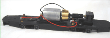
Figure 4 - IHP 87183A chassis' with Bowser Drive & A-line Flywheel.
