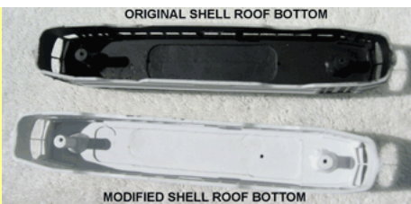
Figure 6 - Shells showing original vs modified milled out roof.
